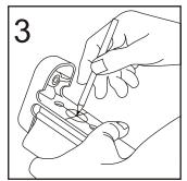
Using a pencil, mark the spot where the 1" hole on the bottom of rail will be drilled. IMPORTANT! Drill the 1" hole first before you drill the 3/8" hole. If not, it is possible that the bit will wobble and create imperfect hole that the 1" bung will not fit properly.
