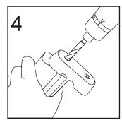
It is necessary to flip the jig during the process. The 1/4" hole side most commonly is drilled into the fitting to accept the lag portion of the bolt. The 3/8 hole is usually drilled on the side where the Railbolt would be tightened into place.
