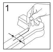
Mark a "center line" about 3" long on each piece on the two sections being joined.
