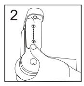
Be sure to align the jig with the "center line" by looking through the windows that are part of the jig. Once lined up perfectly using your hand press the jig firmly into the end cut. It should fit flush against the end.
