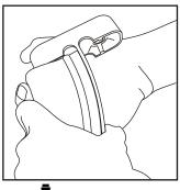
The jig can also be used with an easement. Mark centerline, press firmly into end. Holding the end with one hand and aligning the flap bending it to fit the easement align the holes through the windows in jig. Once lined up, the flap can be released and hole can be drilled. The "positioning pins" will help hold it in proper position to drill hole.
