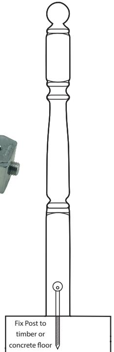
Use a chemical anchor to secure into concrete, the hole must be slightly larger than the screw shaft.
