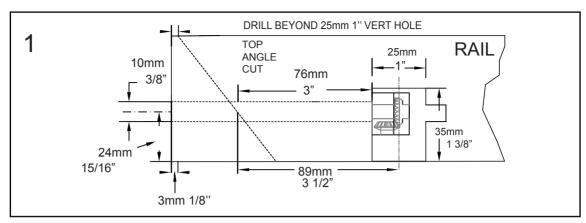
Cut rail 90 degrees square. Then mark proper angle on railing 3mm 1/8" in from end of 90 degree cut. Mark center of rail on 90 degree cut, up 24mm 15/16" from bottom of rail. Drill a 25mm 1" dia. hole in bottom of rail on centerline 89mm 3-1/2" from where the angle and 24mm 15/16 dimension intersect hole, should be 35mm 1-3/8" deep. Drill a 10mm 3/8" dia hole in end of the rail. Hole should be 101mm 4" deep drilling past 25mm 1" hole.
