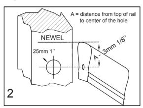
Cut rail at pitch from 3mm 1/8" mark. Measure distance from top of rail to center (A) of 10mm 3/8" hole on pitch (Note the measure) Now, mark a line on the newel that represents the top of pitch cut which is top of the rail. Then measure down the distance from top of rail to center of 10mm 3/8" hole (A) and subtract 3mm 1/8" this is the center of the disc.
