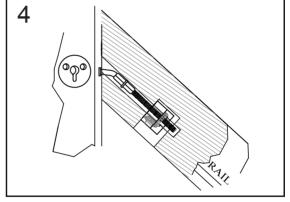
Slide rail on bolt and "Dry Fit" to be sure of proper angle and fit. If another cut is needed take the least amount off to correct cut. The 10mm 3/8" deep hole that was drilled has allowed enough room for you to make this adjustment. Install bolt + gear head. Retract tip as far as you can to angle when sliding into position you may have to extert a small amount off pressure to newel to help slide tip into
