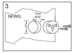
Drill 25mm 1" hole 7mm 9/32" deep Install keyhole dics so that it is flush or slightly under in post. Secure disc with screws. (Tip: Pre drill holes to accept screws)
