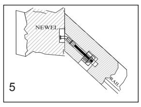
When proper fit is complete, glue, insert angled tip and tighten into place with 5mm driver + ratchet or allen wrench. Glue and insert a wooded 25mm 1" dia. plug. Sand
